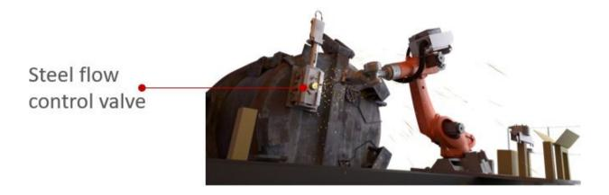
Replacement of the refractory pieces (listed below) includes manual setting of mortar to ensure a good tightness between each of the components. This operation is critical, as a bad sealing results in a major incident (molten steel leakage through the valve).
